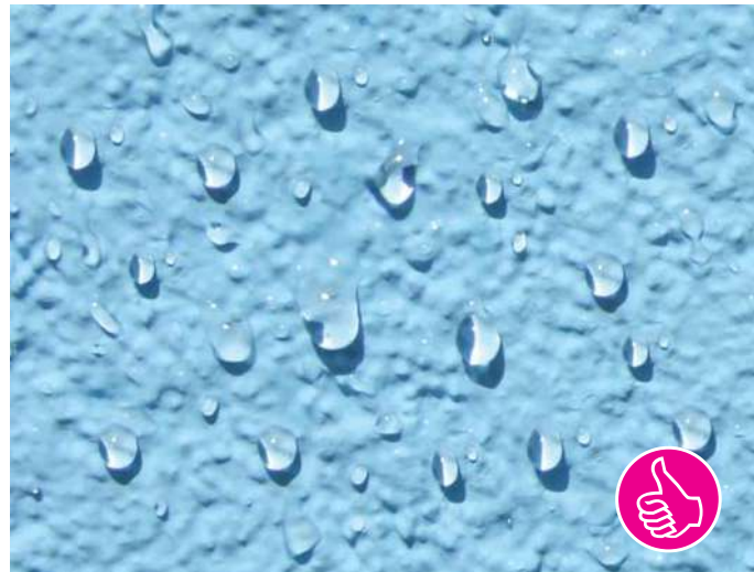
water does not soak into the structure of the paint
