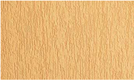
Rustic texture produced with Ceresit CT 35 mineral plaster, grain size 2.5 mm, obtained by circular floating with a plastic float
