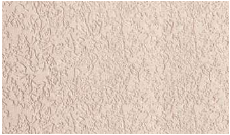
Rustic texture produced with Ceresit CT 35 mineral plaster, grain size 2.5 mm, obtained by circular floating with a plastic float
