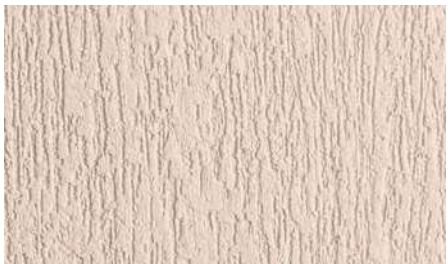
Rustic texture produced with Ceresit CT 35 mineral plaster, grain size 2.5 mm, obtained by floating with a plastic float in one direction
