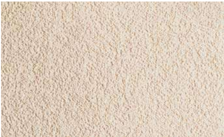
Stone texture produced with Ceresit CT 60 acrylic plaster, grain size 1.5 mm, obtained by floating with a plastic float
