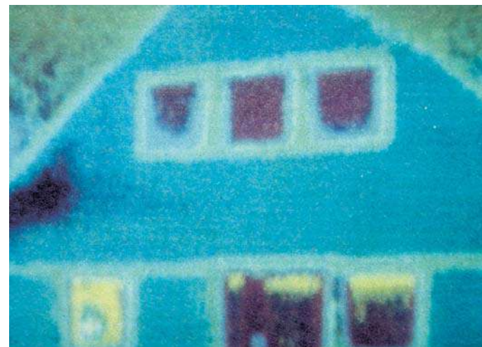
The effect of thermal insulation on a building's external walls is visible in the two thermographic pictures above. In the left picture, the colours yellow and orange mark areas of visible heat loss that can be avoided. Heat flows from the inside of the building, thus raising the temperature of the facade walls. The right picture shows a building whose facade has been thermally insulated. The areas are identical, but they now appear in a blue colour, i.e. they have a much lower temperature due to their thermal insulation. Heat is prevented from flowing from the inside to the outside.
