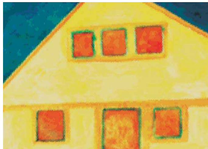
The effect of thermal insulation on a building's external walls is visible in the two thermographic pictures above. In the left picture, the colours yellow and orange mark areas of visible heat loss that can be avoided. Heat flows from the inside of the building, thus raising the temperature of the facade walls. The right picture shows a building whose facade has been thermally insulated. The areas are identical, but they now appear in a blue colour, i.e. they have a much lower temperature due to their thermal insulation. Heat is prevented from flowing from the inside to the outside.
